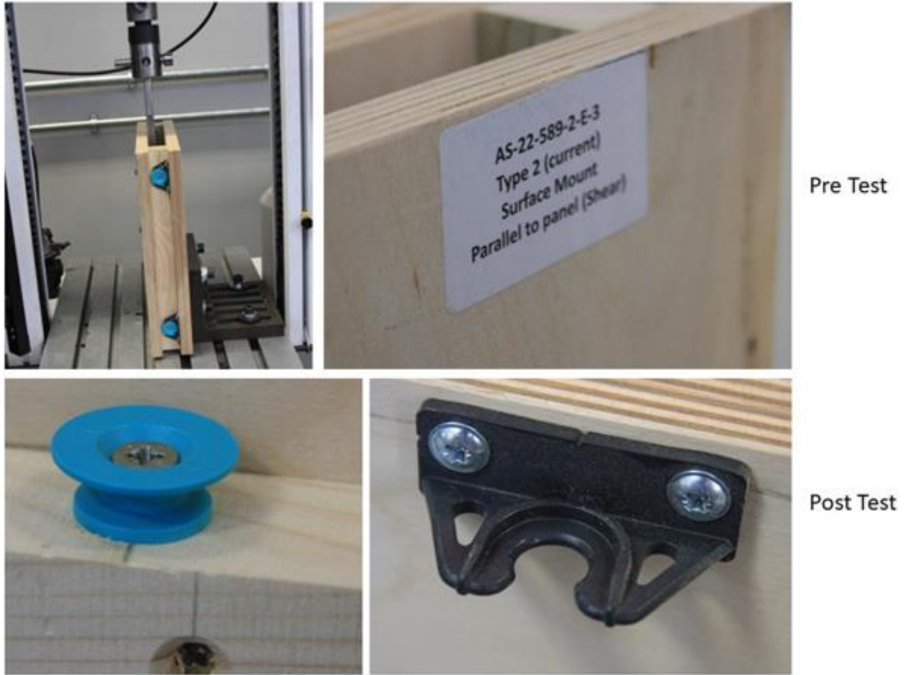
Figure 5.3 Type 2 Shear test images
