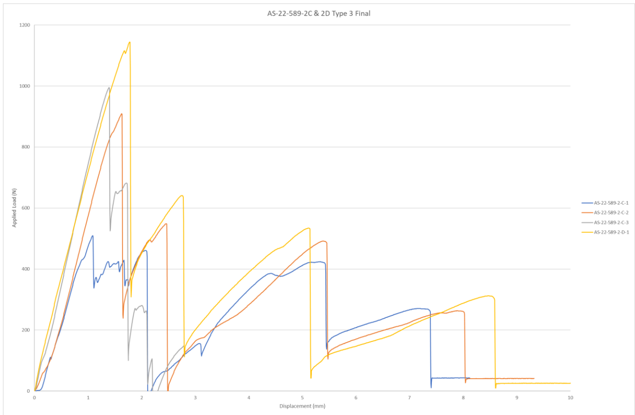
Figure 5.6 Type 3 Perpendicular pull test
