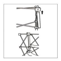
Slot the flat end of the channel bars into the lower hub from the side. Insert the Channel Bar B horizontally to front and back.
