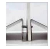
Place the drilled substrate in between the 2 metal base pieces
