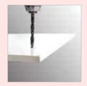
2 Drill the marked holes over the substrate at a minimum of 9mm in diametre
