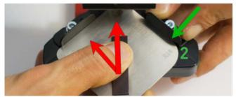
**Push** the alignment tool against the blade and the guide bracket #1. **Move** the **guide bracket #2** over to the alignment tool to adjust its position (see arrows above.)
