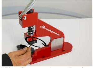
**Tighten** the upper grub screw from the HPS025 again without exerting much force, so that the lever runs smoothly.
