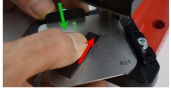
**Push** the alignment tool against the blade. **Move** the **guide bracket #1** over to the alignment tool to adjust its position (see arrows above.)
