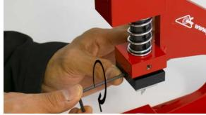
**Align** the upper holder with the HPS025 and fix its position, **tightening** the grub screw of the upper holder.
