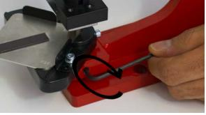
When the alignment from step 7 is done, **tighten** the lower grub screw from the HPS025 to fix the lower holder.
