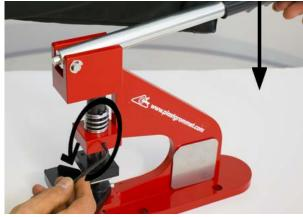
**Holding** the lever, **loosen** the grub screw to leave the lever in the starting position.
