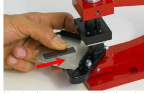
Use the alignment tool pushing it against the guide brackets and the blade. **Move** the lower holder until it is **well adjusted** and there is no space left between the guide brackets and the alignment tool (see picture below.)
