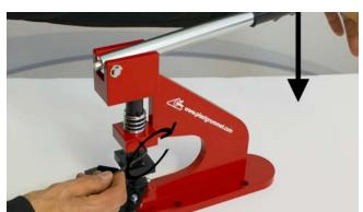
**Press** and keep the lever down, **making** the blade come in contact with the cutting pad; then **tighten** the upper grub screw from the HPS025 to leave the lever blocked (see picture below.)
