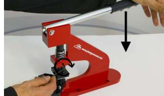
**Press** and keep the lever down, making the blade come in contact with the cutting pad; then **tighten** the upper grub screw from the HPS025 to leave the lever blocked.
