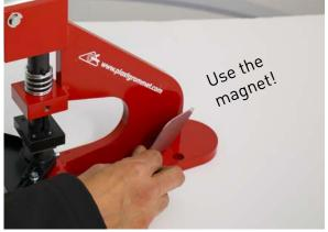
**Put** the alignment tool on the body of the HPS025 for further use.
