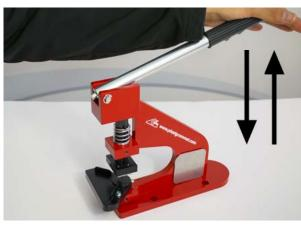
Check that the lever works properly. If it does not run smoothly, adjust the tightening of the upper grub screw from the HPS025.
