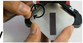
Once the position of the guide bracket #1 is adjusted, **tighten** its screw.
