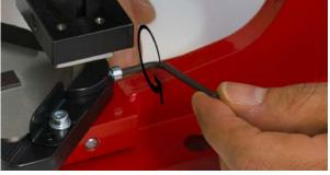
**Tighten** the screw of the cutting pad.
