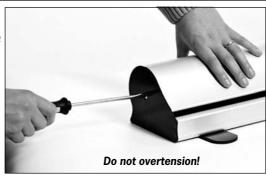
If adjustment is needed, hold the cassette firmly in place then depress and turn the adjusting screw clockwise to increase the tension (the tension mechanism adjusts in halfturn increments). Slowly release pressure on the screw turning slightly counter-clockwise and allow it to again lock in place. If tension has been lost completely, we recommend 20-25 full clockwise turns.
